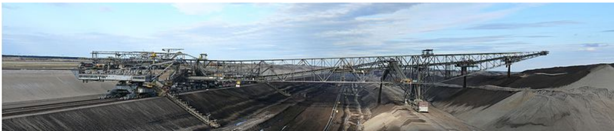
Figure 45. F 60 conveyor bridge in the Jänschwalde mine (Brandenburg, Germany)
