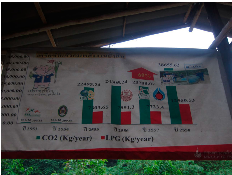
Figure 4. Avoided carbon dioxide and LPG use in Pa Deng due to their biogas systems computed by the Pa Deng moso network. The horizontal axis denotes the year in the Buddhist calendar system, where the year 2558, for example, corresponds to the year 2015 in the Gregorian calendar. Source: Photographed by the author, November 2016.
