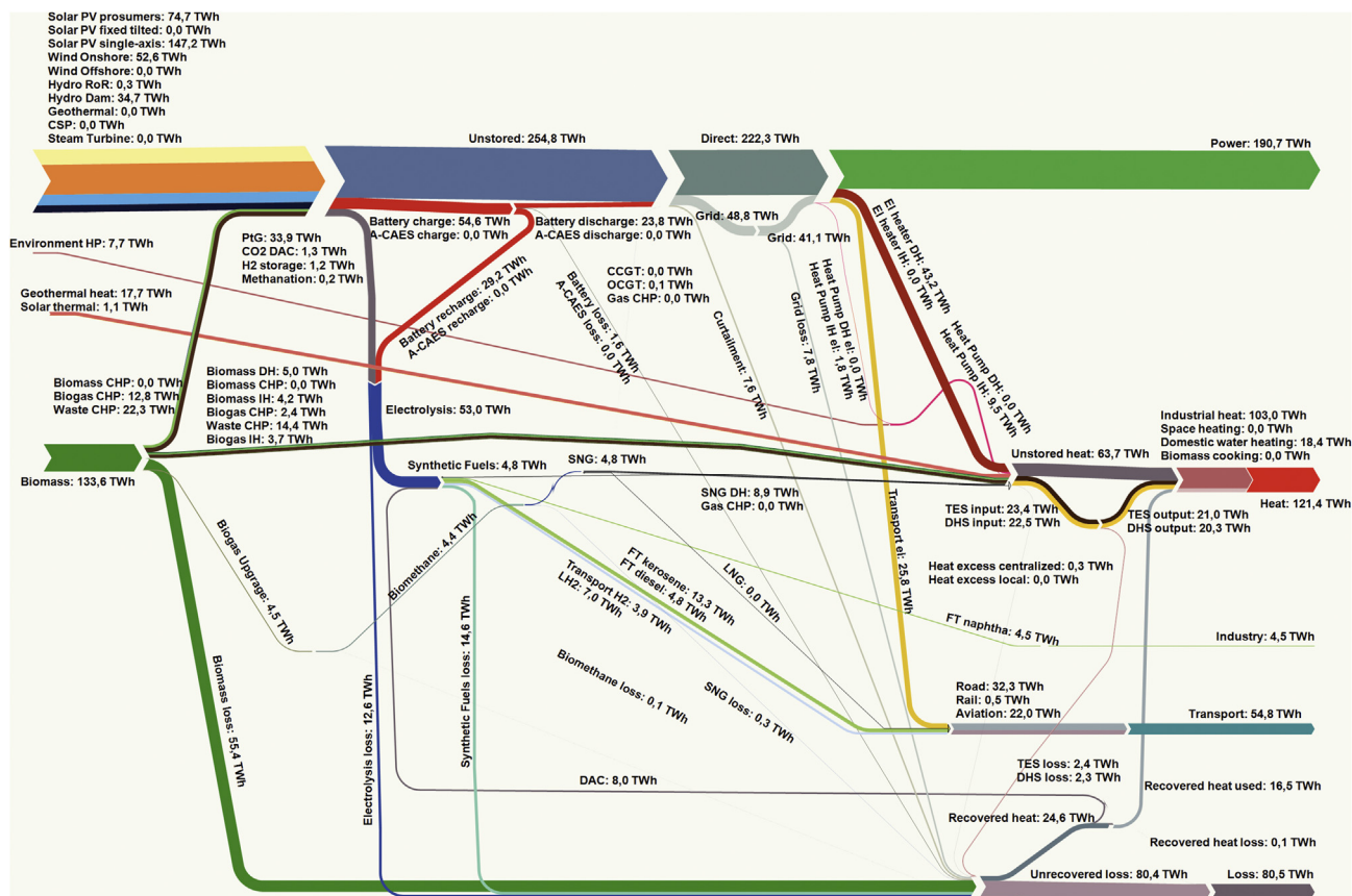
Fig. 21. Energy flow of the system in 2050 for BPS-1. All numbers displayed are in TWh.
