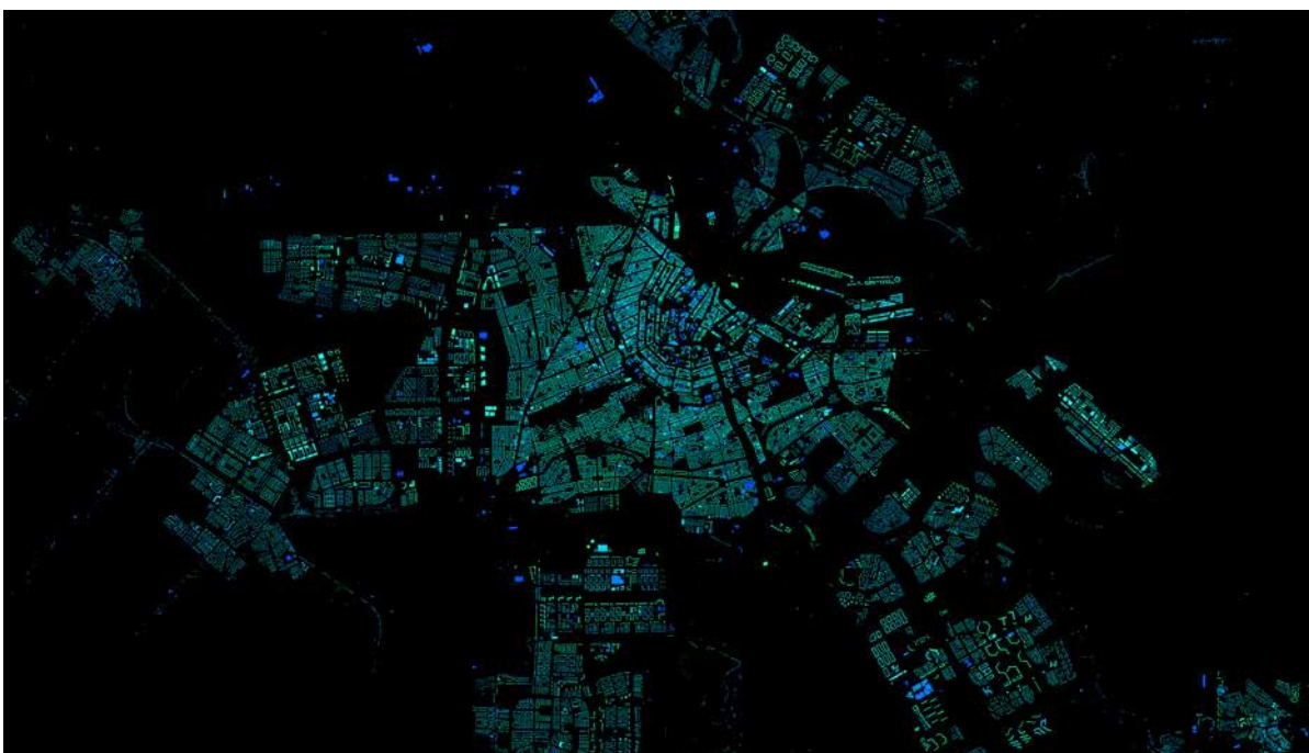
Figure 4.2: Maps of retrievable copper (blue-green) in Amsterdam. Such maps can be used to identify sites with urban mining potential.
