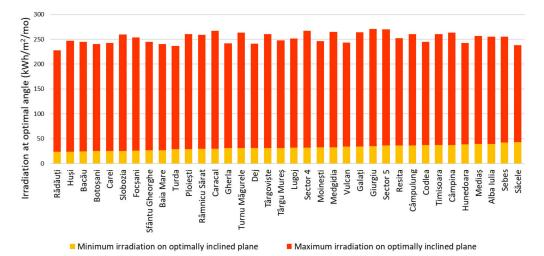
**Figure 13.** The minimum and maximum values of the irradiation at optimal tilt of the PV modules for best mounting angle.
