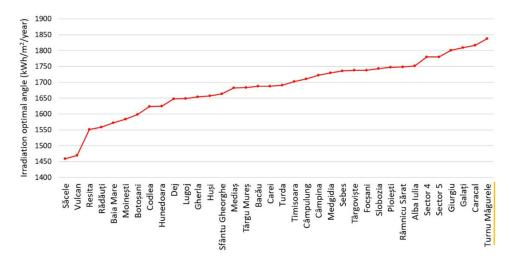
**Figure 16.** Average values of yearly sum of irradiation on optimal tilt of the PV modules for best mounting angle. Source: elaborated by the authors.
